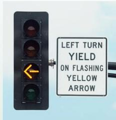
It's a new type of signal placed OVER the left-turn lane at a signalized intersection. The signal display includes a flashing yellow arrow. Other displays on the signal are a steady green arrow, steady yellow arrow and steady red arrow. This Federally approved signal has been successfully tested in other states and will be installed in Ohio and nationwide in the near future.
